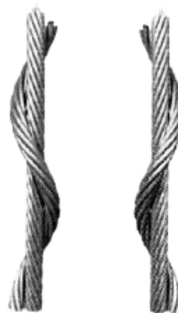
Fig. 11 Left Hand Lang's Lay
