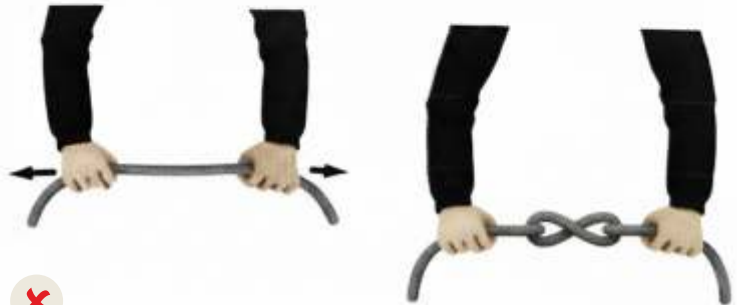
Fig. 32 : The Wrong Way to Remove a kink in Wire Rope
