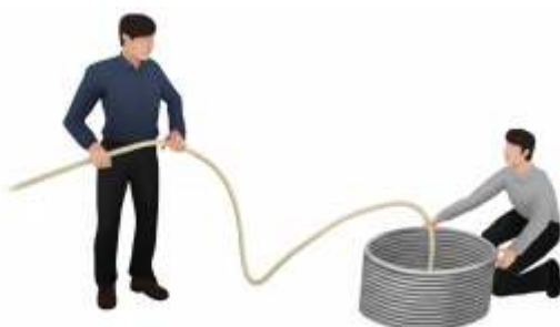
Fig. 27 : Running Out a Coiled Down Wire
