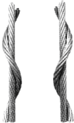
Fig. 7 Left Hand Lay Rope
