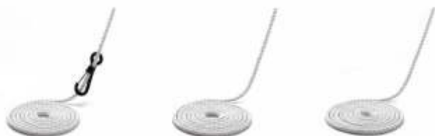
Fig. 24 : To Coil a Rope Running
