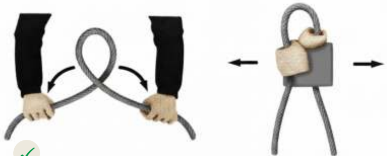
Fig. 31 : The Right Way to Remove a kink in Wire Rope
