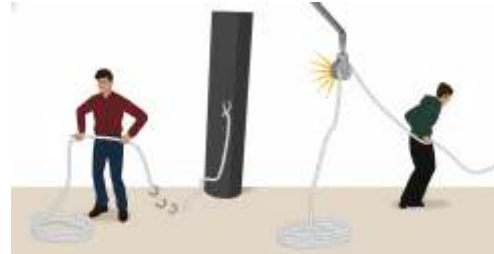
Fig. 22 : Mistakes in Coiling Down
