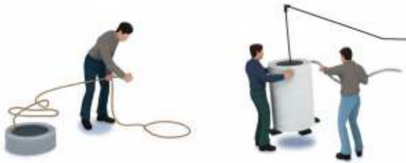
Fig. 25 : Opening a New Coil
